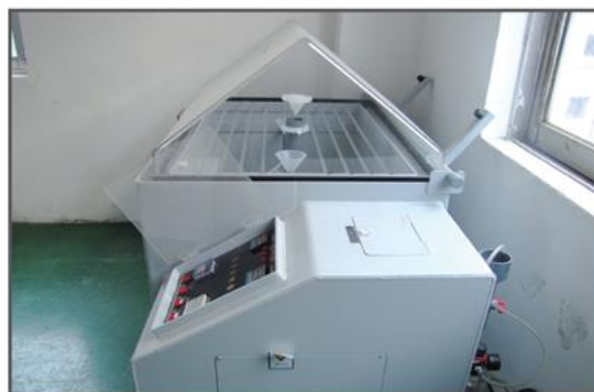
盐雾测试仪 (Salt mist testing system) Test the salt mist performance of Waterproof fan with level IP55 and IP68
